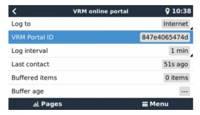
Check 'Last contact'. If this shows dashes or a time that is much larger than 'Log interval', the CCGX is not able to contact the VRM database.
