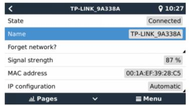
When using Ethernet and State shows 'Unplugged', verify that the Ethernet network cable is not faulty: try another one. The two lights at the back of the CCGX, where the Ethernet RJ45 cable plugs in, should be lit or blinking. Two dead lights indicate a connection problem.
